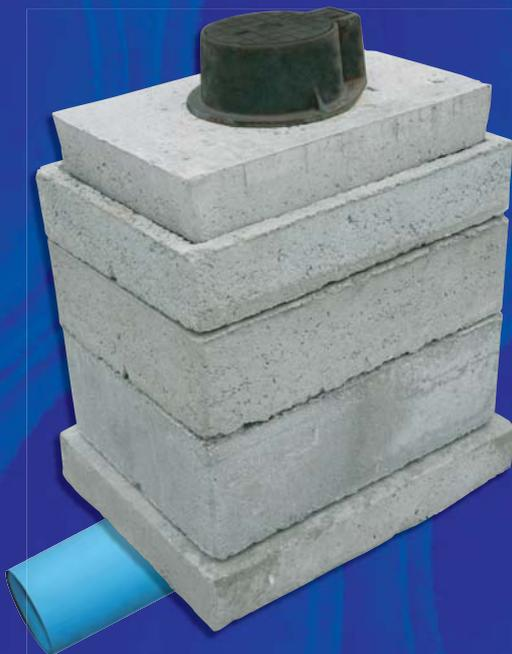
From the assembled box sections shown, you can see how the bases and covers are used. The base has a 225mm diameter hole in the centre, which allows the valve to come up through into the inspection chamber. The box sections are then built to the desired height using the various heights available.
